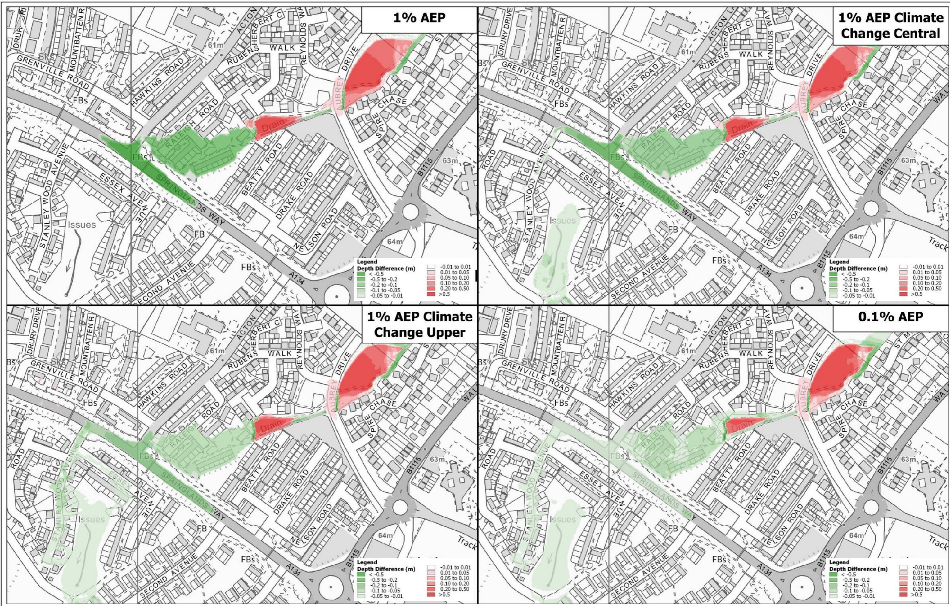
Figure 5-7 Aubrey Drive: Flood Depth Difference, 1% AEP to 0.1% AEP Storm Events
