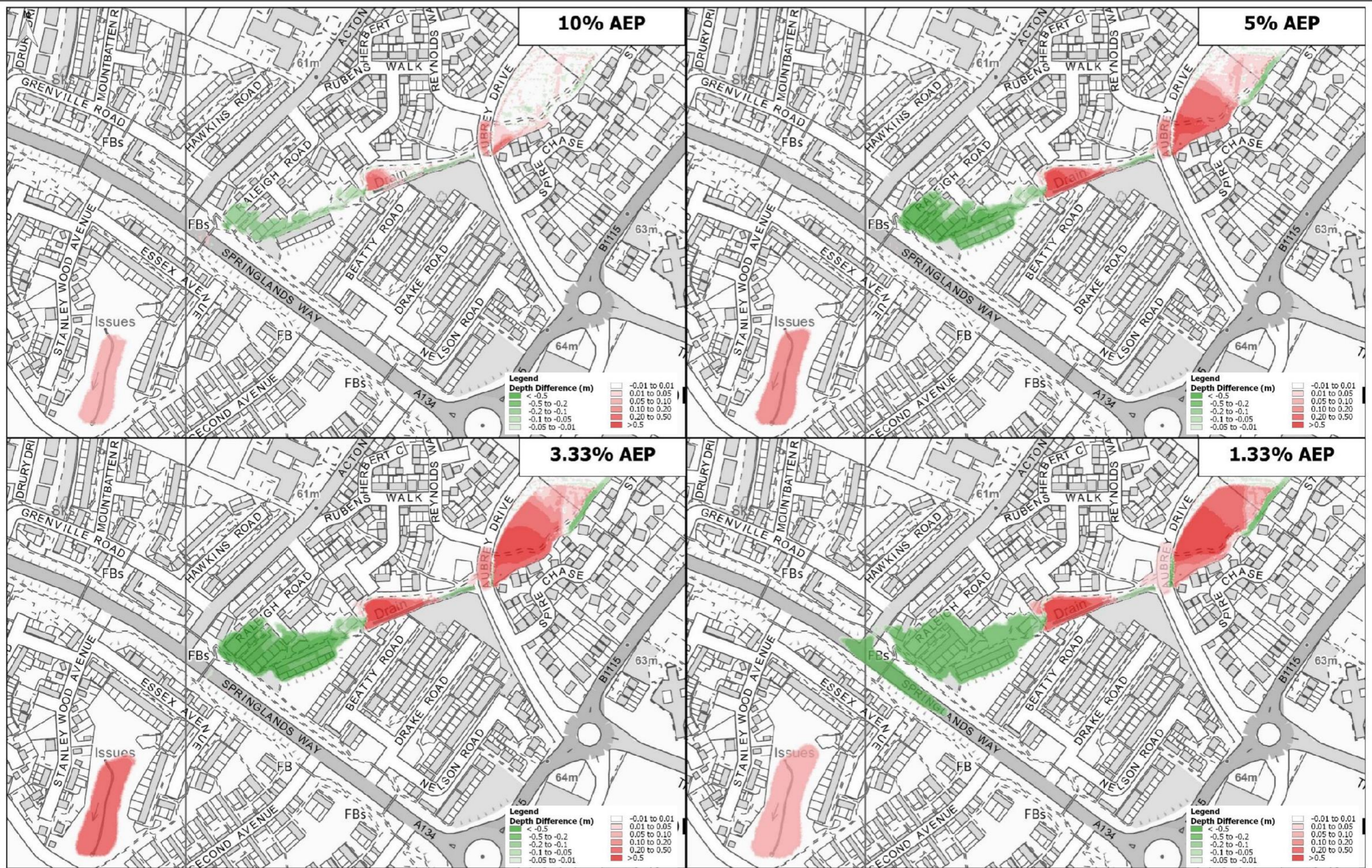
Figure 5-6 Aubrey Drive: Flood Depth Difference, 10% AEP to 1.33% AEP Storm Events
