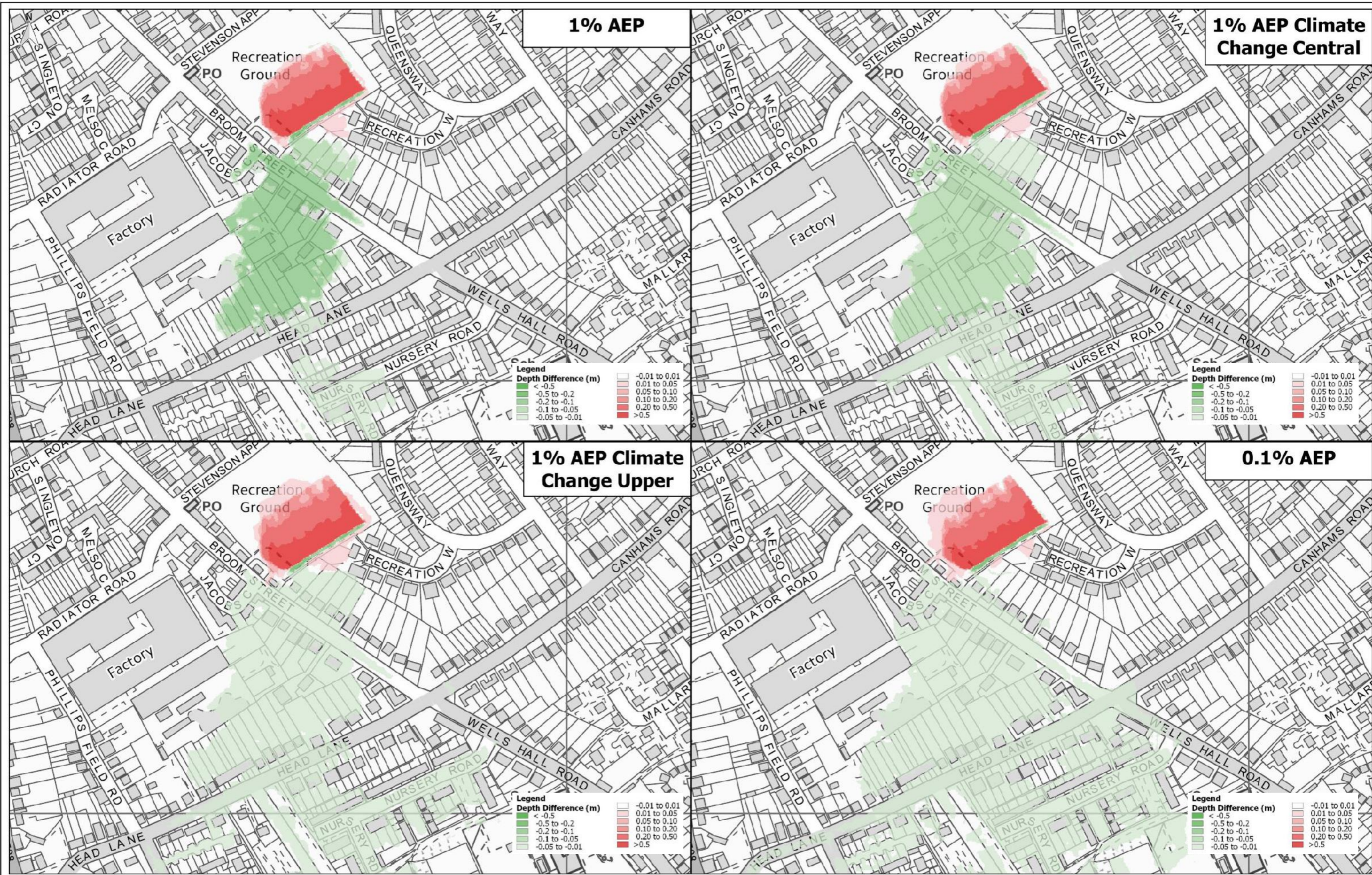
Figure 5-13 Great Cornard Recreation Ground: Flood Depth Difference, 1% AEP to 0.1% AEP Storm Events
